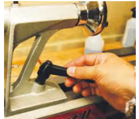
▲ A well-positioned lock makes tailstock adjustments very easy
